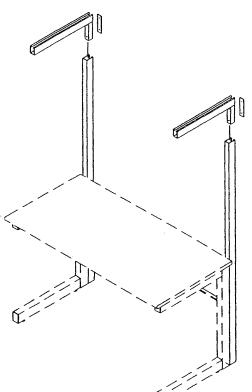
Shelves are available in Painted Steel or Wire. Metal Shelves have a 1 5/8" lip that extends 1/2" above the shelf surface. In a level position, the shelf lip is located in the back and serves as a backstop. In an inclined position (invert brackets), the shelf lip is located in the front and serves as a gravity stop. The shelf lip can be used to hang parts bins. Mounting brackets are included.
